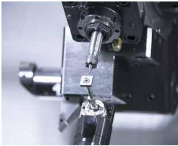
Quick and accurate tool calibration can be done by contacting the tool tip with the sensor. This process is done easily with the use of M-Code and the calibration process takes roughly 30 seconds.
